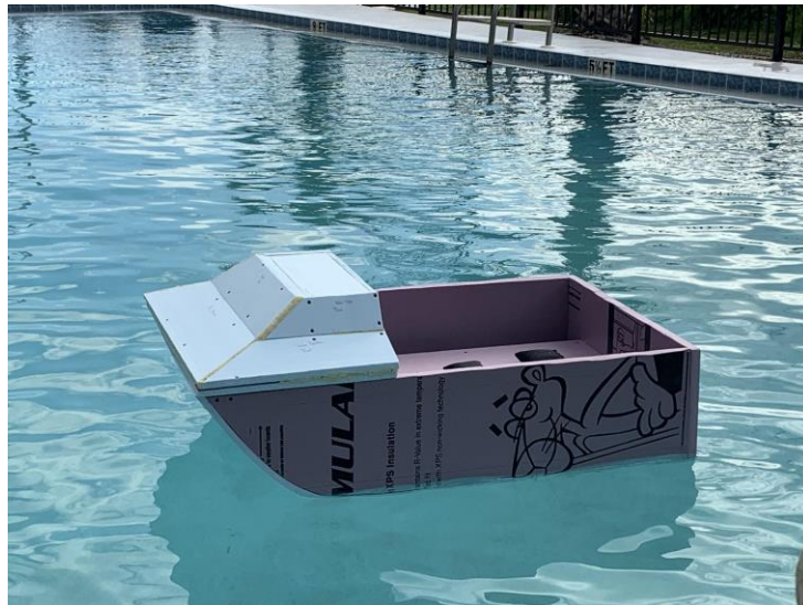
Image 11-The boat mold floating with 12 lbs of weight applied
